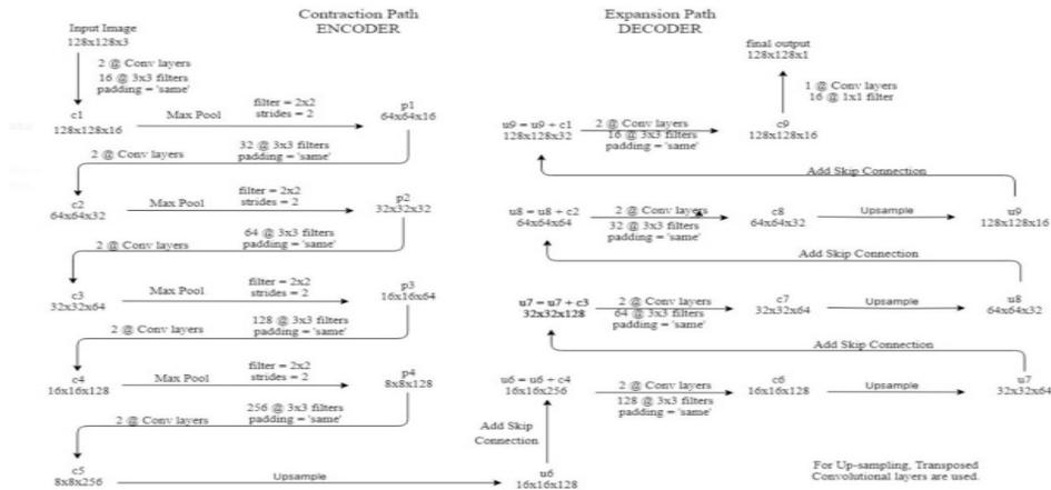
Figure.3: Modified UNET architecture
