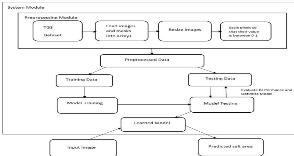
**Figure1:** System Architecture for Salt Identification in Seismic Images
