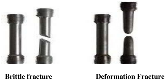
Fig. No.1 Visual representation of shape changes during tensile testing
