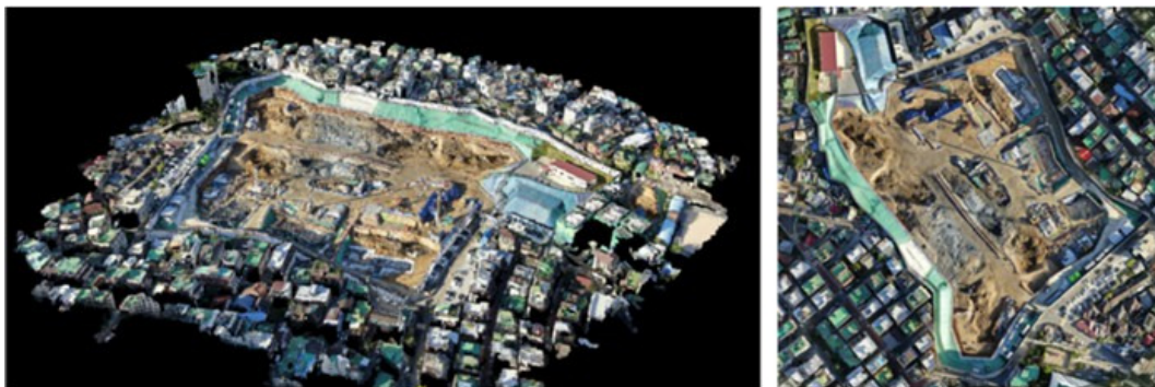
Figure 2: Drone data processing results of 3D point cloud (left) and orthomosaic (right) [21]
