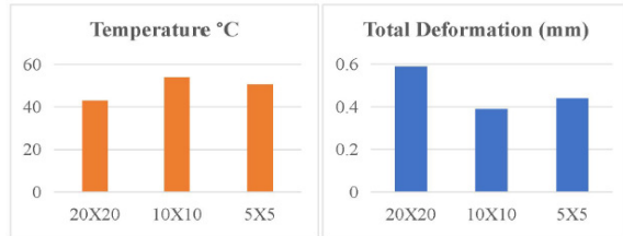
Figure8. Temperature & total deformation of three different lattice structures.
