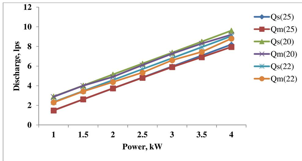
**Fig. 5.** Comparison of the simulated and measured pump discharge
