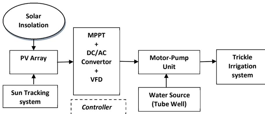
**Fig.2. Block diagram of solar PV operated trickle irrigation system**
