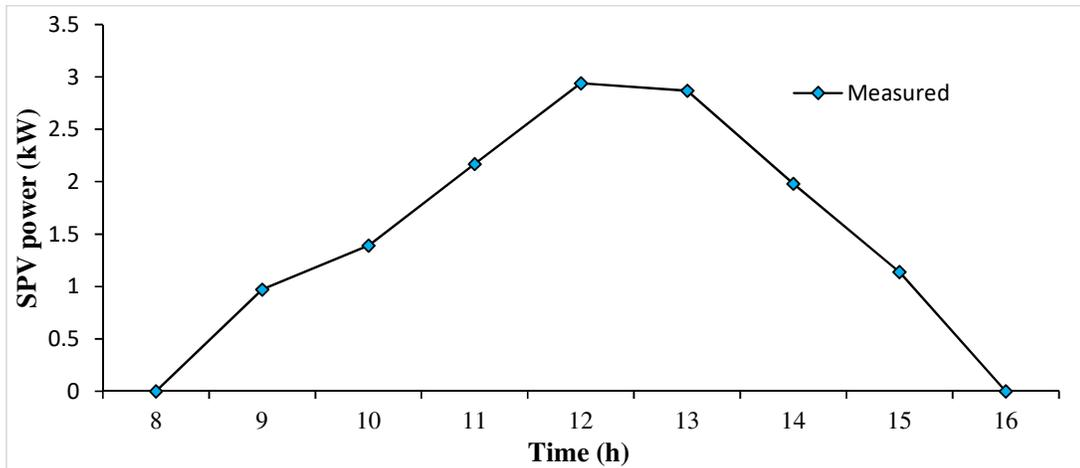
**Fig. 4. Average measured solar PV power output**
